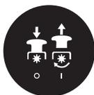
Lift the blade engagement button up to engage. Press the blade engagement button down to disengage.
